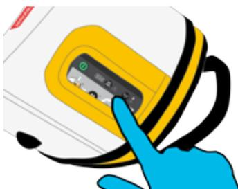
To minimise interruptions, having a charged spare LUCAS battery in the carrying case is always recommended. When the battery gets low during operation, it can be replaced by a new one without turning the device off. To change the battery during operation:
